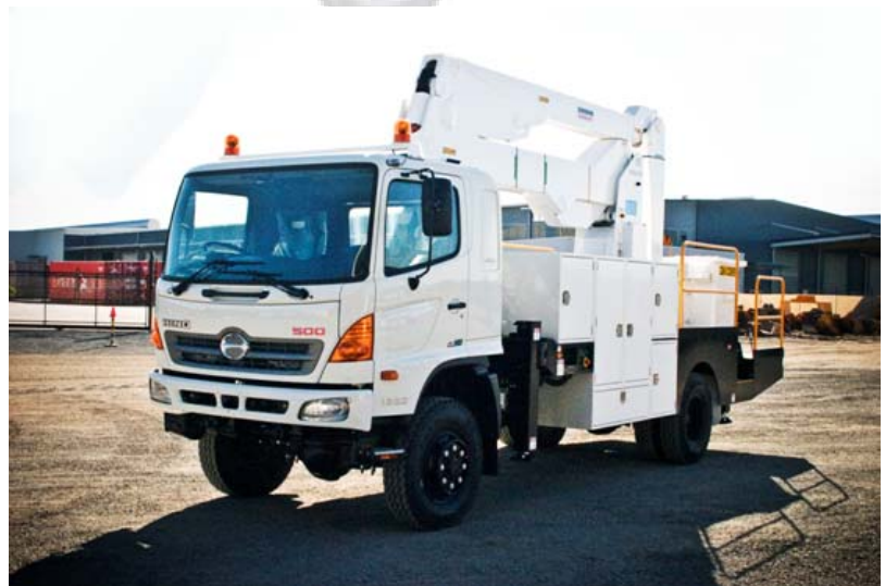
Below: Sherrin Equipment 18M Glove and Barrier Travel Tower - Series II in the Brisbane yard, mounted to a Hino Truck.
